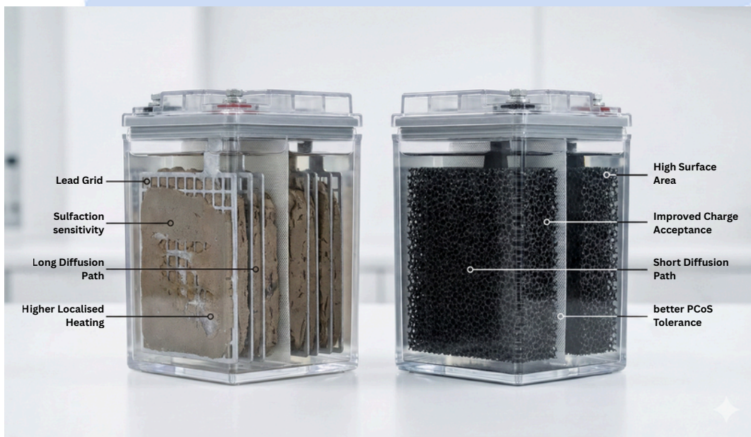
Figure 2. Schematic comparison: conventional grid + paste vs 3D carbon-foam scaffold.
